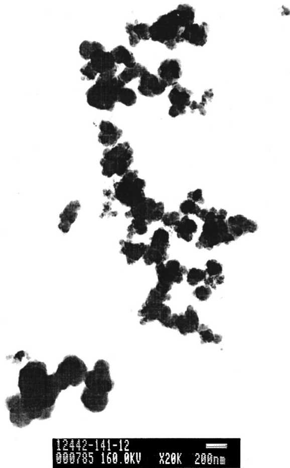
Fig. 3 TEM data obtained in the plume of a 10 cm diameter D_4 fire
